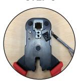
Place the new blade onto the crimper, and use the Phillips screwdriver to tighten it.
