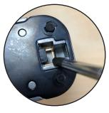
Turn to the other side of the tool, take the tool up, and use the front end of the screwdriver to knock the trimming blade a couple times, so the trimming blade could come off the tool a little bit.
