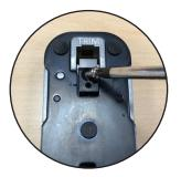
Loosen the screw of the trimming blade.
