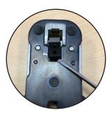
Turn to the original side of the tool, use the flathead screwdriver to force the trimming blade to come off completely.
